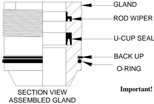
**Important!** Be sure all gland and piston seals have been installed correctly before cylinder is assembled!
