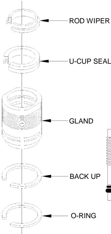
All gland seals shown with a section removed to facilitate correct installation.
