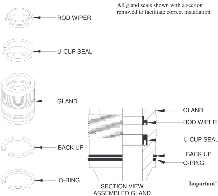
All gland seals shown with a section removed to facilitate correct installation.
