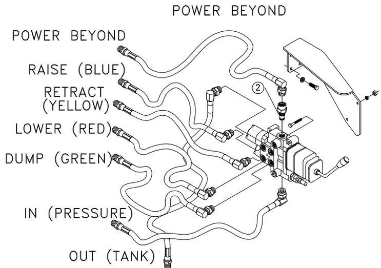
For closed center applications item one (655445) is replaced by item two (673097) and item one is installed in item two.
