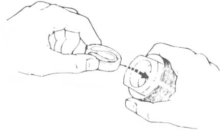
**Important!** Be sure all gland and piston seals have been installed correctly before cylinder is assembled!
