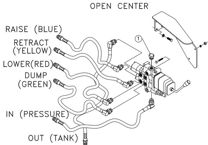
For power beyond applications item one (673096) plug, must be removed and item two (673097) power beyond sleeve must be added.
