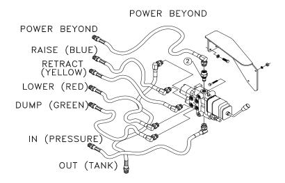
For closed center applications item one (655445) is replaced by item two (673097) and item one is installed in item two.
