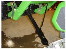
1. Raise loader frame slightly to permit loader stand reengagement. (Fig 10-1)
