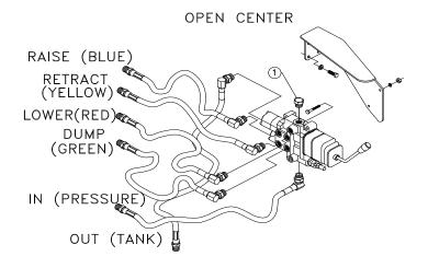
For power beyond applications item one (673096) plug, must be removed and item two (673097) power beyond sleeve must be added.
