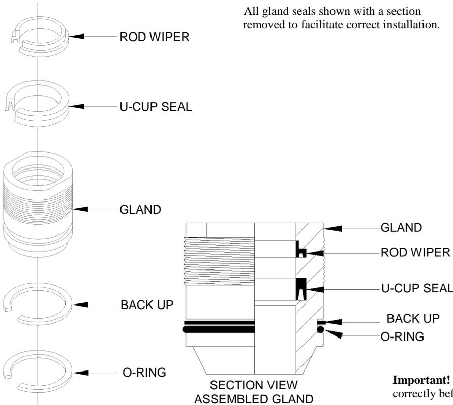
Note: To install rod wiper and U-cup seal, fold similar to shape shown below, slip into gland bore and locate each in its respective groove. Tools are used to fold seals, take care not to damage sealing surfaces.
