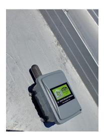
Head Space Monitor is mounted on the outside of the roof. Mount one as close to the center of the bin as possible to monitor the peak air under the roof.
