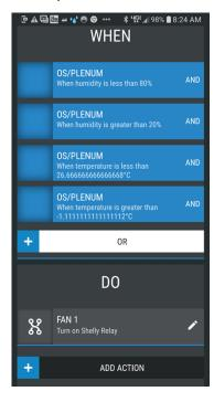
Fan will run when the humidity is between 80% and 20% and when the temperature is between 26.6 celuis (80 degree F) and -1.1 celuis (30 F).
