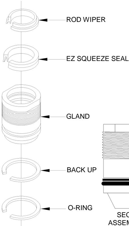
All gland seals shown with a section removed to facilitate correct installation.
