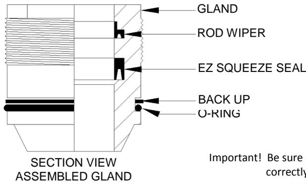
Important! Be sure all gland and piston seals have been installed correctly before cylinder is assembled!
