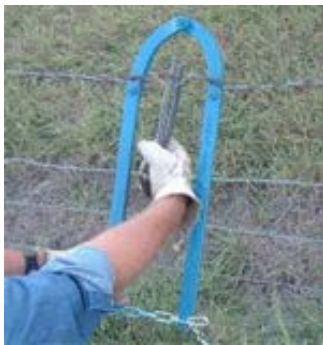
Step 5. Inset tool handle into the loop. Wrap the loop around the spare wire.
