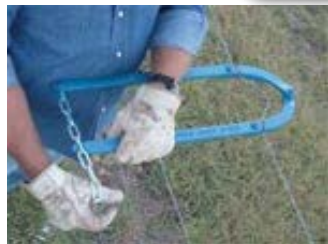
Step 2. Bring the handles together to stretch the wire as tight as possible.
