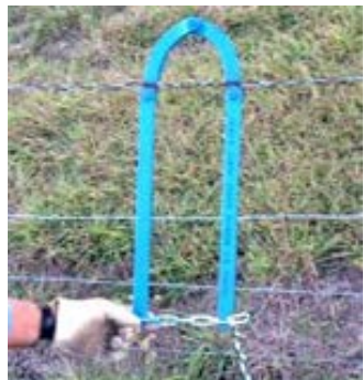
Step 6. Loosen the chain and remove tool from wire.
