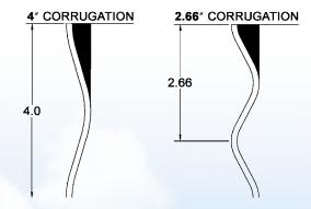
**4" corrugated sidewall sheets** provide better vertical load carrying capacities. While unloading, grains flow easily down the bin wall with less resistance.
